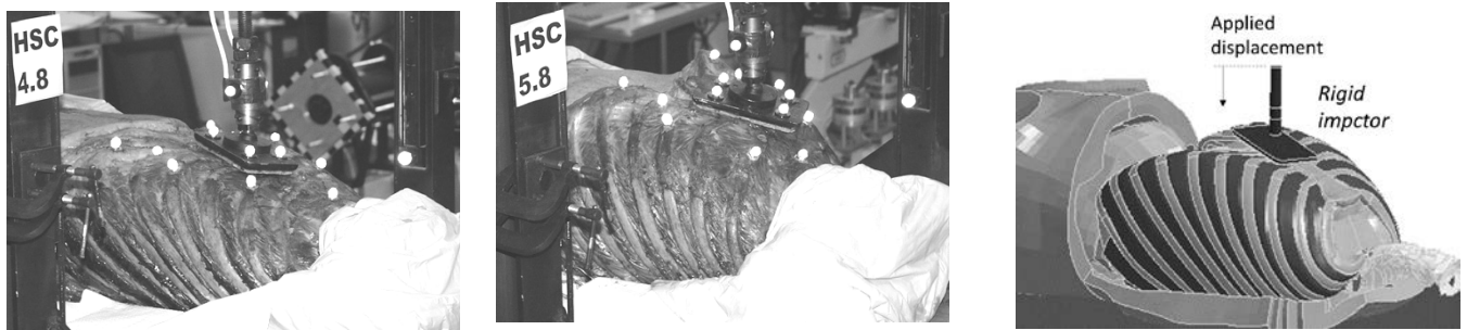
Fig. 3. Denuded thorax indenter impacts at mid sternum (centre located at Rib 5). Left : pre-test 4.8 (adopted from [35]). Middle : pre-test 5.8 (adopted from [35]). Right : corresponding simulation model setup. The location of the strain gauges is roughly on one line along the edge of the denuded flesh.
