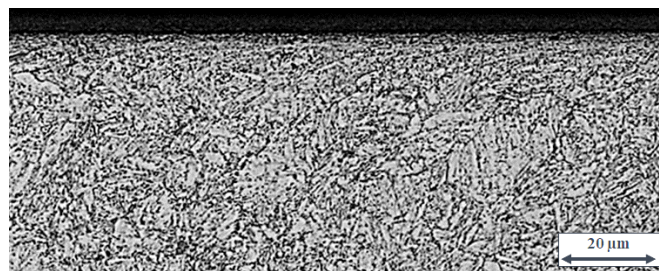
Fig. 7 AISI4140 QT 600, v_c = 300 m/min, f = 0.3 mm and a_p = 1.2 mm
