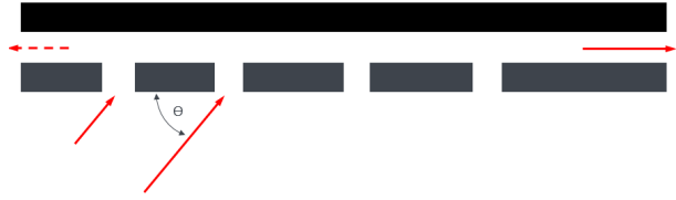
Figure 6. Schematic of the coupling from OCCWG cross section to the fundamental mode waveguide behind the mirror surface. The waveguide depth is matched for the single hole contributions to coherently add up.
