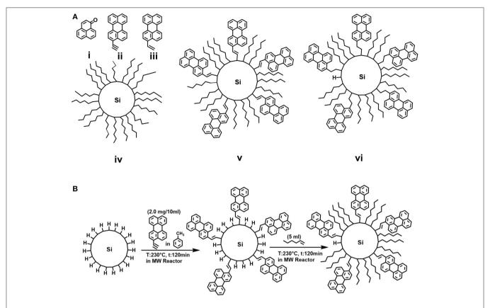
FIGURE 1 | (A) Molecular structures of (i) phenalenone (phe), (ii) 3-ethynylperylene (dye-1), (iii) 3-ethenylperylene (dye-2), (iv) hexyl-functionalized SiNCs (C6-SiNCs), (v) 3-ethynylperylene/hexyl-functionalized SiNCs (C6-2-SiNCs); (B) Schematic representation of the hydrosilylation reaction of hydrogen-terminated SiNCs with dye and 1-hexene.
