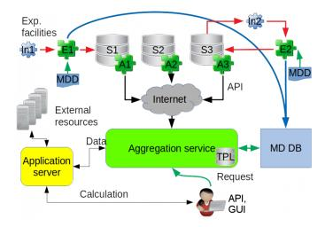
Figure 1. Scheme of the joint data life cycle architecture by GRADLCI. Here Si stand for local data storages, Ini represent data sources of different types, MDD is a metadata description, Ei are metadata extractors, Ai are adapters that provide APIs for the data access, TPL is a template library, and MD DB is the metadata database.
