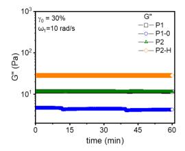
**Figure 9.7:** Time-dependent tests for the thiol-ene (P1) polymer, oxidized thiol-ene polymer (P1-O), the ADMET polymer (P2), and the hydrogenated ADMET polymer (P2-H) at 150 °C with  $\gamma_0 = 30\%$ ,  $\omega_1 = 10$  rad/s.
