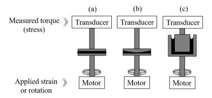
**Figure 4.2:** Schematic illustration of (a) parallel-plate, (b) cone-plate and (c) Couette geometry in a strain-control rheometer. The motor is located at the bottom and applies defined deformation to the sample (the black part in between geometries) via the lower geometry. The torque transducer measures the resulting mechanical response and it is connected to the upper geometry.
