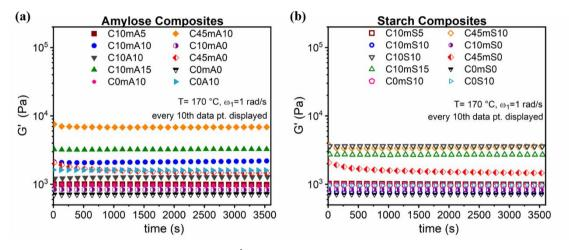
Figure 8.5: Time dependency of the G' at 170 °C with  $\omega_1 = 1$  rad/s in the linear viscoelastic regime for the neat LDPE and the composite samples.
