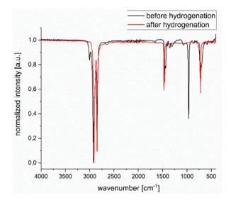
Figure A3: IR-Spectrum of polycyclooctene before and after hydrogenation.
