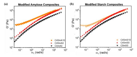
**Figure 8.8:** The  $G'(\omega_1)$  as a function of the  $\omega_1$  at  $T_{ref} = 150$  °C via TTS for neat LDPE and LDPE composites containing 45 wt% cellulose (C) and 10 wt% of (a) modified amylose (mA), and (b) modified starch (mS).
