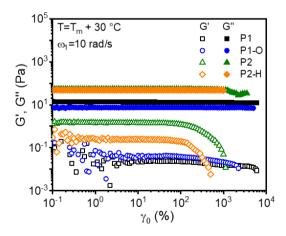
**Figure 9.6:** Strain amplitude ( $\gamma_0$ ) dependency tests for the thiol-ene (P1) polymer, oxidized thiolene polymer (P1-O), the ADMET polymer (P2), and the hydrogenated ADMET polymer (P2-H) at  $T_m + 30$  °C,  $\omega_1 = 10$  rad/s.
