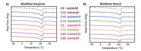
*Figure A2:* DSC results of samples containing (a) modified amylose and (b) modified starch compatibilizer and their respective reference samples.
