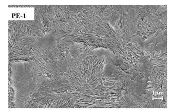
Figure 6.54: The SEM image of the PE-1 (see Chapter 6.3.2) quiescently crystallized.
