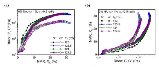
Figure 6.9: (a) Correlation of dynamic moduli (G', G'') and crystallinity  $X_C$  and (b) vice versa.
