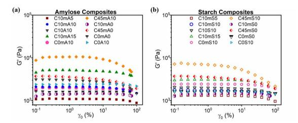
**Figure 8.3:** The G' as a function of the  $\gamma_0$  at 150 °C and  $\omega_1 = 1$  rad/s for the neat LDPE and the composite materials with cellulose (C), (a) modified and non-modified amylose (A) compatibilizer and (b) modified and non-modified starch (S) compatibilizer.
