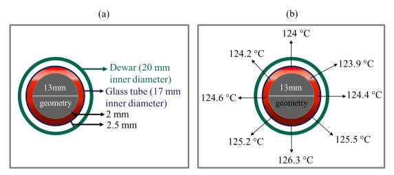
*Figure 5.7:* Illustrated inside view of RheoNMR setup from the top shows that (a) the pieces with inner diameter and distance in between pieces and (b) the measured temperature gradient in the sample chamber which causes temperature inhomogeneity across sample volume.
