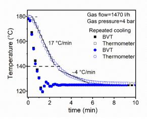
*Figure 5.13:* The temperature change during the time in the BVT unit and the thermometer. The BVT thermocouple was positioned at the outer part of the glass tube which holds probe coils (see Figure 5.12). The thermocouple of the thermometer was placed inside of the special upper geometry as touching the sample from the center. Cooling was divided into two regions with rates of cooling = 17 °C/min and critical cooling = ~4 °C/min.
