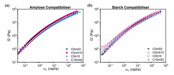
**Figure 8.6:** The G' as a function of the  $\omega_1$  at  $T_{ref} = 150$  °C was plotted via TTS for neat LDPE and LDPE composites containing 10 wt% cellulose (C10mA/S0) or composites with 10 wt% of (a) modified amylose (mA) or non-modified amylose (A), and (b) modified starch (mS) or non-modified starch (S).
