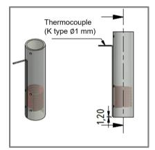
*Figure 5.12:* The designed fixed thermocouple to outer to the glass tube which holds the probe coil. The design and the plot were done by Karl-Friedrich Ratzsch.
