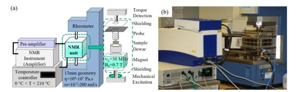
*Figure 5.4:* (a) Illustration and (b) a photograph of the RheoNMR setup taken from Ratzsch et al. 2017. The BVT unit is the temperature controller.
