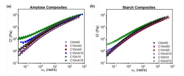
**Figure 8.7:** The G' as a function of the  $\omega_1$  at  $T_{ref} = 150$  °C was plotted via TTS for neat LDPE and LDPE composites containing 10 wt% cellulose (C) with 5-15 wt% of (a) modified amylose (mA), and (b) modified starch (mS).
