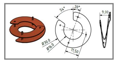
*Figure 5.8:* The designed and plotted vortex creator by Karl-Friedrich Ratzsch. Dimensions are in mm size.
