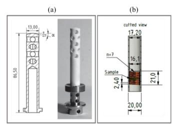
*Figure 5.2*: (a) Drawing and the photo of the machinable ceramic cone geometry for rheometer which has 13 mm diameter and 86.50 mm length. It has holes for fast thermal stabilization. (b) Illustration of the probe coil (length 21 mm N = 7 turn) is in a glass tube with an inner diameter of 17.2 mm. Adapted from Ratzsch et al. (2017).
