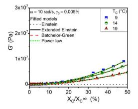
**Figure 7.8:** Correlation of the G' and the  $\frac{X_C(t)}{X_C^{\infty}}$  for temperature dependent experiments with fitted suspension models up to 50% of the  $\frac{X_C(t)}{X_C^{\infty}}$  as represented lines: black dot line for Einstein model, black line for extended Einstein, red dash line for Batchelor-Green, green short dot line for power-law models.
