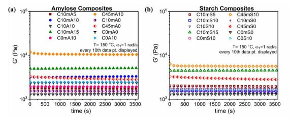
Figure 8.4: Time dependency of the G' at 150 °C with  $\omega_1 = 1$  rad/s in the linear viscoelastic regime for the neat LDPE and the composite samples.
