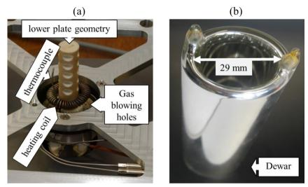
*Figure 5.3:* (a) Photo of the lower geometry, that is surrounded by a heating coil. Nitrogen gas is blown from the bottom holes. The thermocouple measures the temperature of the sample chamber. (b) Dewar is used to insulating the magnet to avoid frequency drifts due to changes in the temperature of the magnet.
