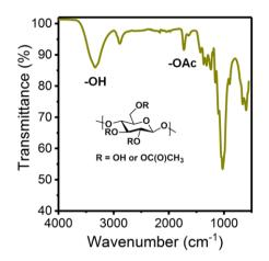
*Figure A1: FT-IR* spectrum of cellulose obtained by the acetic acid extraction of wood chips clearly showing absorption in the carbonyl region as a result of acetylation during extraction.
