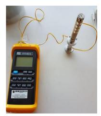
Figure 5.9: Photograph of the special upper geometry with the connected thermocouple.
