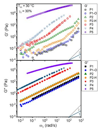
**Figure 9.8:** Frequency-dependent measurements for the thiol-ene (P1) polymer, oxidized thiolene polymer (P1-O), the ADMET polymer (P2), hydrogenated ADMET polymer (P2-H), HDPE samples P3, P4, and P5 at  $T_m + 30$  °C,  $\gamma_0 = 30\%$ .
