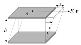
*Figure 4.1: Two-plate model for the shear experiment. Material is located between two plates in a distance h. The upper plate with the area A is moved by the force F over a distance x.*
