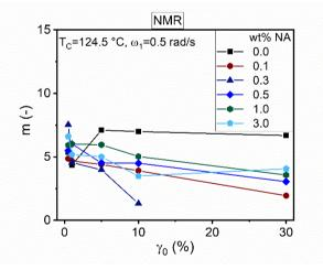
*Figure 6.38:* Foubert exponent ( $m_{NMR}$ ) for neat HDPE and HDPE/NA blends from the data of the NMR part of the RheoNMR.
