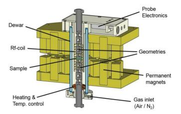
*Figure 5.1:* Schematic overview of used Halbach magnet with the NMR probe of the RheoNMR setup and the rheometry counterparts. Adapted from Ratzsch et al. (2017).
