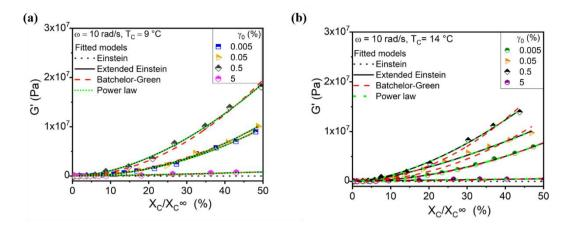
**Figure 7.9:** Correlation of the G' with the  $\frac{X_C(t)}{X_C^{\infty}}$  for varying  $\gamma_0$  at (a)  $T_C = 9$  °C, and (b)  $T_C = 14$  °C. with fitted suspension models up to 50% of the  $\frac{X_C(t)}{X_C^{\infty}}$  as represented lines: black dot line for Einstein model, black line for extended Einstein, red dash line for Batchelor-Green, green short dot line for power-law models.
