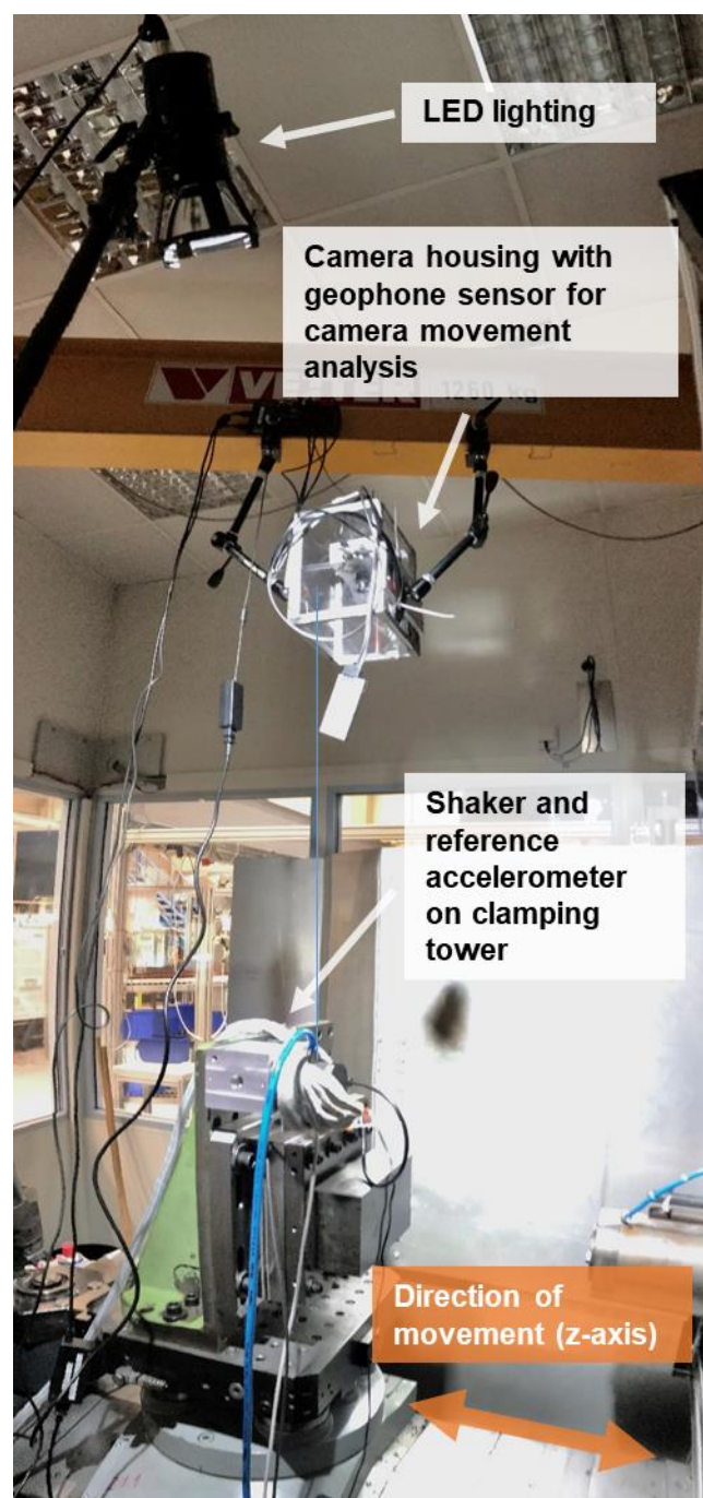
Fig. 1. Setup overview with camera filming moving clamping tower with attached shaker.
