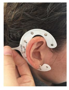
FIGURE 8.1: cEEGrid - A Flexible EEG Array With Ag/AgCl Electrodes That Can Be Placed Around the Ear Using Adhesives.
