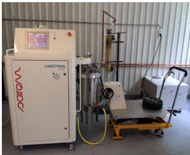
Figure 4: Pilot for the extraction of rose essential oil from fresh petals, 2.45 GHz, up to 6 kW, 20 L reactor
