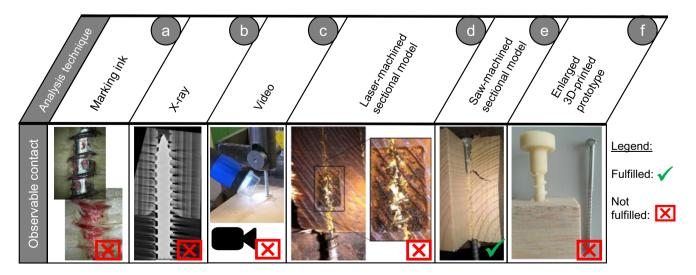
Fig. 3 Application of analysis techniques to the wood screw connection for evaluation of the requirement observable contact
