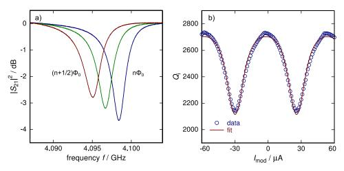
FIG. 3. (a) Transmission curve  $|S_{21}|^2(f)$  of channel 4 for three different values of the magnetic flux threading the SQUID loop. (b) Magnetic flux dependence of the intrinsic quality factor of the resonator of channel 4 as well as a fit assuming a small subgap resistance of the Josephson junction.
