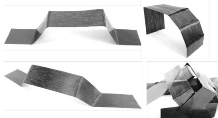
Fig. 2: Possible tape geometries of single tapes and a joined reinforcement.
