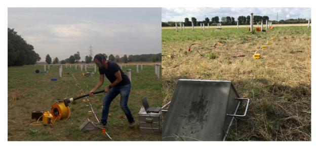
Figure 7.6: Overview of the field conditions and the acquisition layout, along with the prismatic source and its operation towards the inline component (direction of the receiver array).
