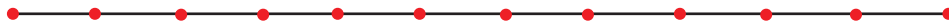
(b) A step-size too small will waste CPU time by performing an unnecessary amount of computation, hence negatively affect the performance. In extreme cases, it also introduces and accumulates unnecessary numerical error.
