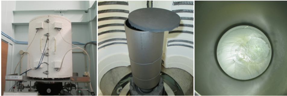
Figure 4. From left to right: a high-temperature oven for NaI(Tl) crystals growth; the graphite crucible; detached NaI(Tl) crystal inside of the graphite crucible after cooling down.
