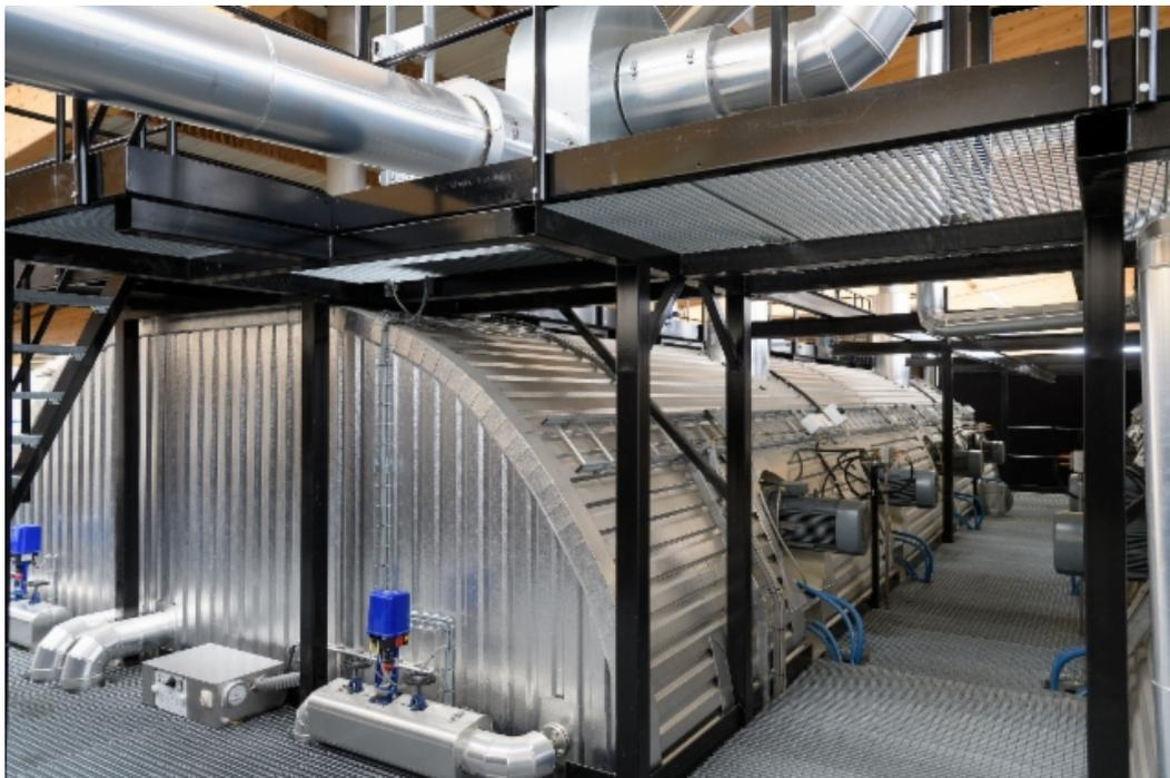
Figura 2.8: Reator de ThermoWood [6].
