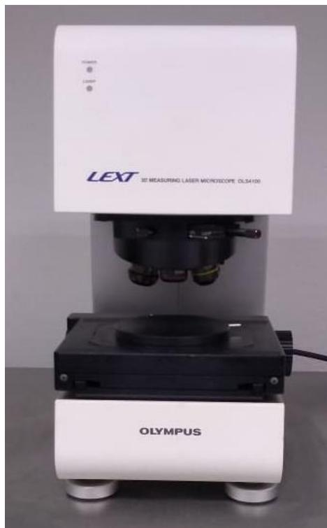
Figura 3.7 - Microscópio confocal Lext 3D measuring laser
