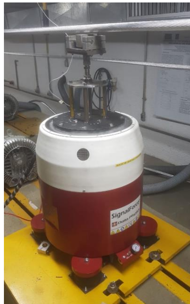
Figura 4-5: Shaker SignalForce Inertial Shake DataPhysics V4dolt.
