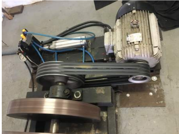
Figure 61 – Brake Disc Machine Pulley System
