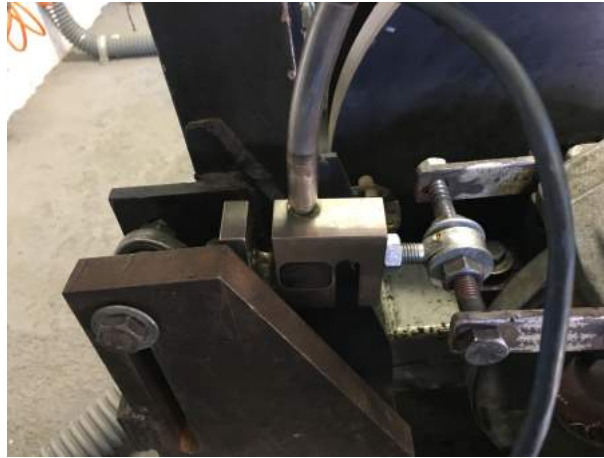
Figure 64 – Load Cell Installed
