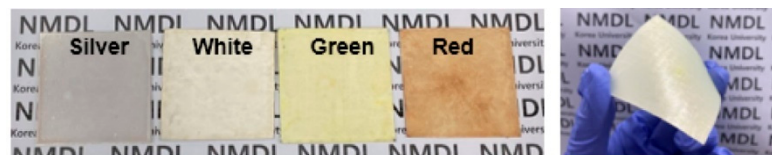
Figure 11. Samples of colored daytime RC emitter researched by Son et al. [111] (reprinted from Nano Energy, Son et al., Colored emitters with silica-embedded perovskite nanocrystals for efficient daytime radiative cooling, 105461, Copyright (2020), with permission from Elsevier).
