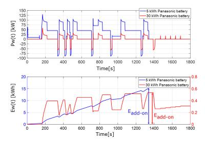
Fig. 13. Power and energy evaluation of the add-on device for Panasonic 5 kWh and 30 kWh batteries, strategy iii, category II.
