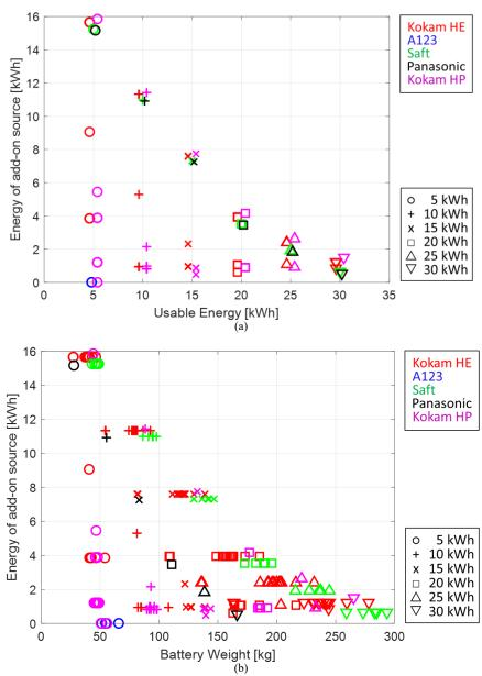
Fig. 14. Energy of the add-on device for strategy iii, category II with respect to (a) usable energy and (b) battery weight.
