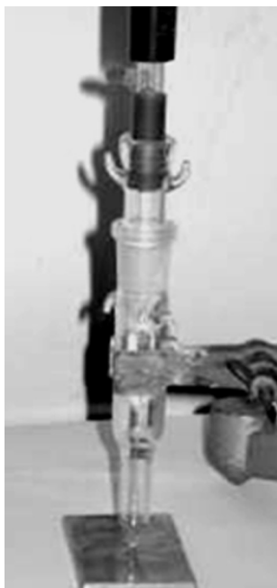
Figure 2. SCE with double mantle for IGC testing by E_{corr} measurements in a drop of the test solution.
