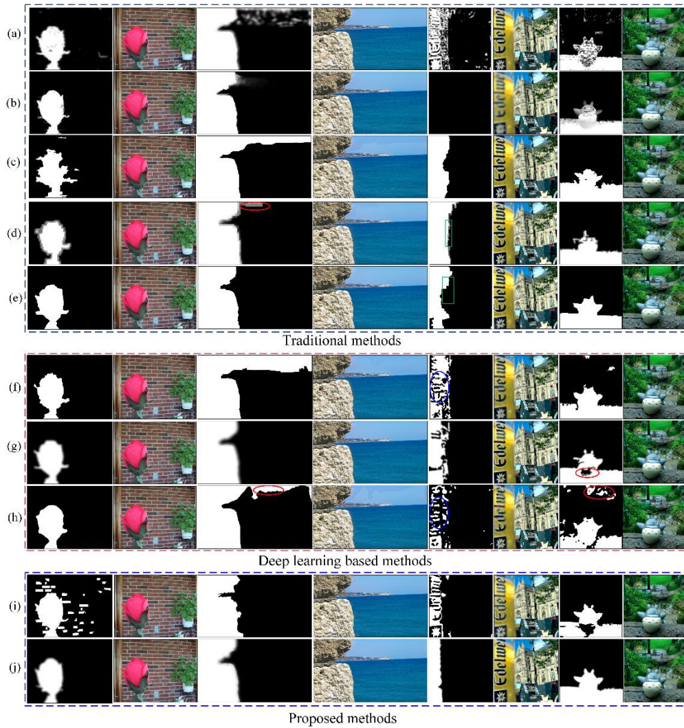
452 453 Fig. 13. Some fusion results on SMD Dataset. (a) GFF; (b) IM; (c) SPixel; (d) LR_RSR; (e) SRCF; (f) p_CNN; (g) CNN; (h) 454 EN_CNN; (i) ULRR without post-processing steps; (j) ULRR. The decision maps in (h) and (i) are initial ones without using any 455 post-processing steps. The remaining decision maps are the final ones after the post-processing steps.
