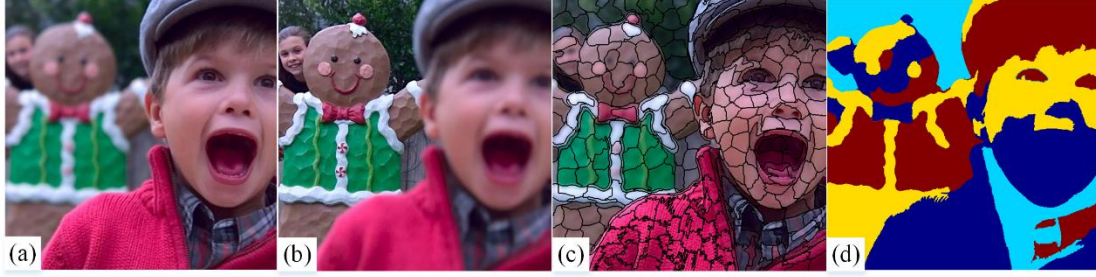
202 Fig. 4. Super-pixel clusters. (a) and (b) Source images with focus on the front and the back, respectively; (c) Results of super-pixel 203 segmentation; (d) Results of super-pixel clustering. 204
