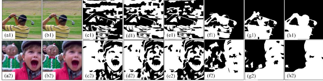
389 Fig. 8. Fusion results by using different dictionaries. (a1) and (b1) A pair of source images with focus on the front and the back, 390 respectively; (c1) ~ (h1) Initial focus decision maps for (a1) and (b1) obtained by using \mathbf{D}_{Ksvd}^{Global} , \mathbf{D}_{Ksvd}^{Ave} , \mathbf{D}_{Ksvd}^{Blur} , \mathbf{D}_{PCA}^{Global} , \mathbf{D}_{PCA}^{Ave} 391 and \mathbf{D}_{PCA}^{Blur} , respectively; (a2) ~ (h2) Another pair of source images and their initial focus decision maps obtained by using different 392 dictionaries. 393
