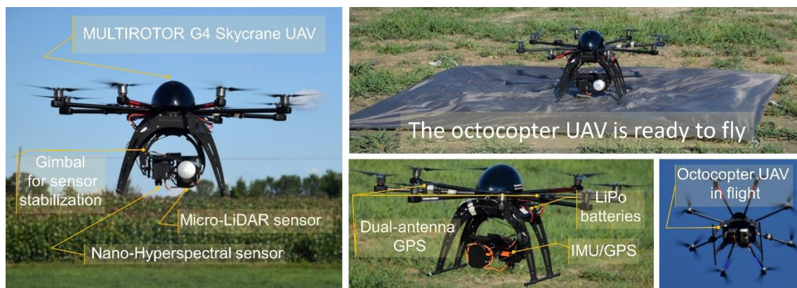
Figure 2. The unmanned aerial vehicle (UAV) platform used for field phenotyping of Arundo donax on the ground and in flight.
