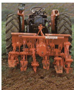
Slika 4. Rotacioni ašov u radu, [15] Figure 4. Rotary wash in operation, [15]
