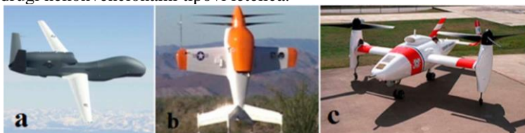
Slika 2. Neki važniji tipovi UAV dronova: (a) HTOL, (b) VTOL, (c) tilt-rotor UAV, [8]. Figure 2. Some important UAV tipe of drones:(a)HTOL, (b) VTOL, (c)tilt-rotor UAV,[8].
