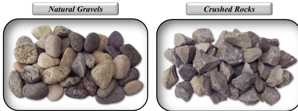
Fig. 4. Natural gravels and crushed rocks widely used as coarse aggregates in concrete which are displayed for visual comparison between real and virtual aggregates exemplified in Table 1 and Fig. 3 .
