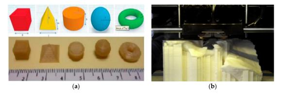
**Figure 4.** (a) 3D representation and images of the 3D geometries printed using the FDM process [38]. (b) 3D printing of an acetabulum through Fused Deposition Modelling (FDM) with acrylonitrile butadiene styrene (ABS) polymer [39]. Reprinted with permission from References [38,39]. Copyright 2017, Elsevier, and 2016, Elsevier.
