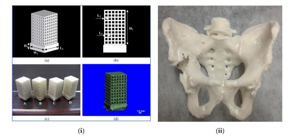
**Figure 5.** (i) (a) Schematic diagram of scaffold model PHBV (diametric view), (b) scaffold model (Side view), (c) scaffold models from Selective Laser Sintering (SLS): (A) PHBV, (B) CaP/PHBV, (C) PLLA, (D) CHAp/PLLA. (d) MicroCT image of a CaP/PHBV scaffold [47]. (ii) A life-size 3D printed model of a patient's pelvis used in providing visual and tactile aid to the surgeon [8]. Reprinted with Permission from Ref. [8]. Copyright 2017, Hindawi Limited.
