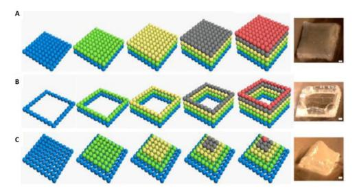
**Figure 3.** Formation of scaffolds fabricated through inkjet 3D printing of alginate hydrogels through varying geometries: (**A**) square model (**B**) pyramid model and (**C**) scale bar. (1 mm) [1]. Reprinted with permission from Ref. [1]. Copyright 2015, John Wiley, and Sons.
