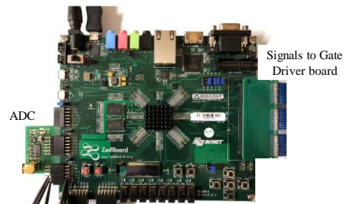
Fig.7 FPGA with ADC to generate gate signals output.
