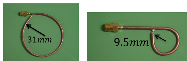
Figure 5 Fabricated loop sensors
