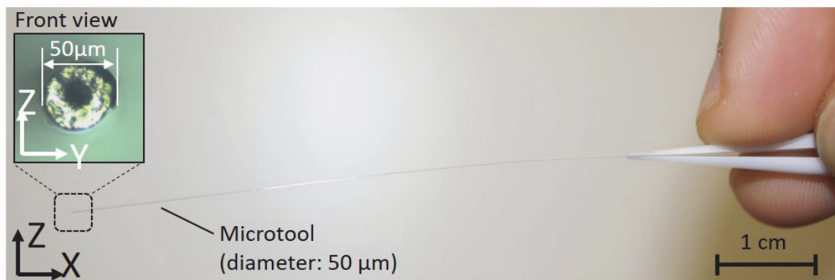
Figure 3.8: An overview of the microtool (tubular structure) with a diameter of 50 \mu\text{m} .
