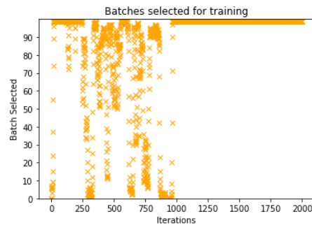
Figure 4. Actions generated by the policy of an unconstrained DDPG teacher on the CIFAR-10 dataset. Orange is the first output (where to select data from) and blue is the second output (how much data to include in the batch). If the batch selected is near zero then this is low entropy data and if it is near the top of the batch selection then this is high entropy data.
