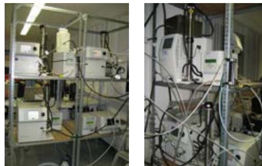
Fig. 1. In this figure it is possible to see the five SMPSs used during the instrument intercomparison.
