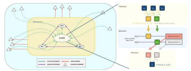
**Figure 2.** Architecture with QML neural networks (Adapted from Asfaw et al., *Learn Quantum Computation Using Qiskit*, 2020, Section 4.1.5 Hybrid Quantum-Classical Neural Networks with PyTorch and Qiskit)
