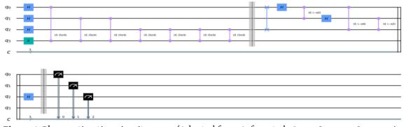
**Figure 4:** Phase estimation circuit source (Adapted from Asfaw et al., *Learn Quantum Computation Using Qiskit*, 2020, Section 3.8 Quantum Phase Estimation)
