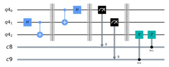
**Figure 3:** Teleportation quantum circuit (Adapted from Asfaw et al., *Learn Quantum Computation Using Qiskit*, 2020, Section 3.2 Quantum Teleportation)
