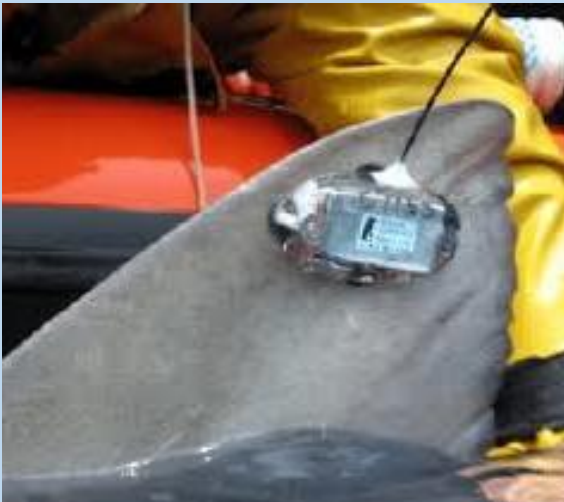
A shark's GPS tracking device on its dorsal fin.
