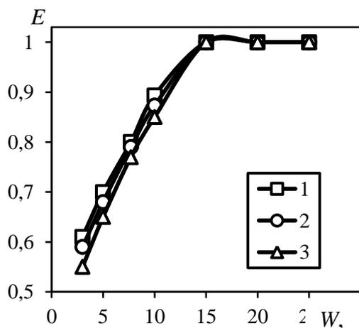
**Figure 3.** Catching efficiency of fine-dispersed particles from gas at different types of elements: 1 – double-T-shaped; 2 – arc-shaped; 3 –  $\Pi$ -shaped. The density of fine particles  $\rho_a = 1000 \text{ kg/m}^3$ .
