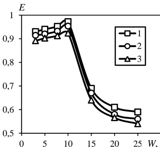
**Figure 4.** Catching efficiency of fine-dispersed particles from gas at different types of elements: 1 – double-T-shaped; 2 – arc-shaped; 3 –  $\Pi$ -shaped. The density of fine particles  $\rho_a = 2000 \text{ kg/m}^3$ .
