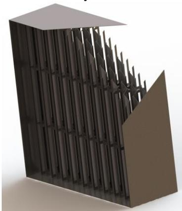
**Figure 1.** A three-dimensional model of the rectangular separator with double-T-shaped elements.
