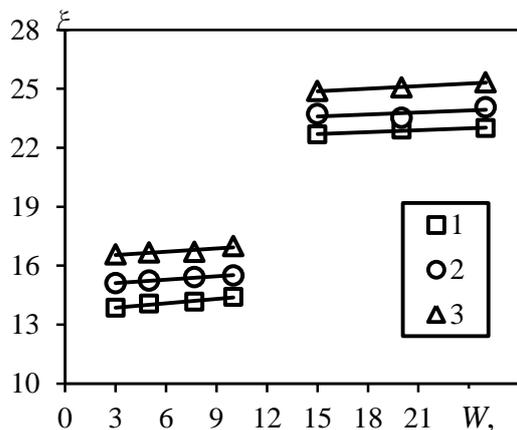
**Figure 2.** Relationship between hydraulic resistance coefficient and inlet gas flow velocity at different types of elements: 1 – arc-shaped; 2 – double-T-shaped; 3 –  $\Pi$ -shaped.
