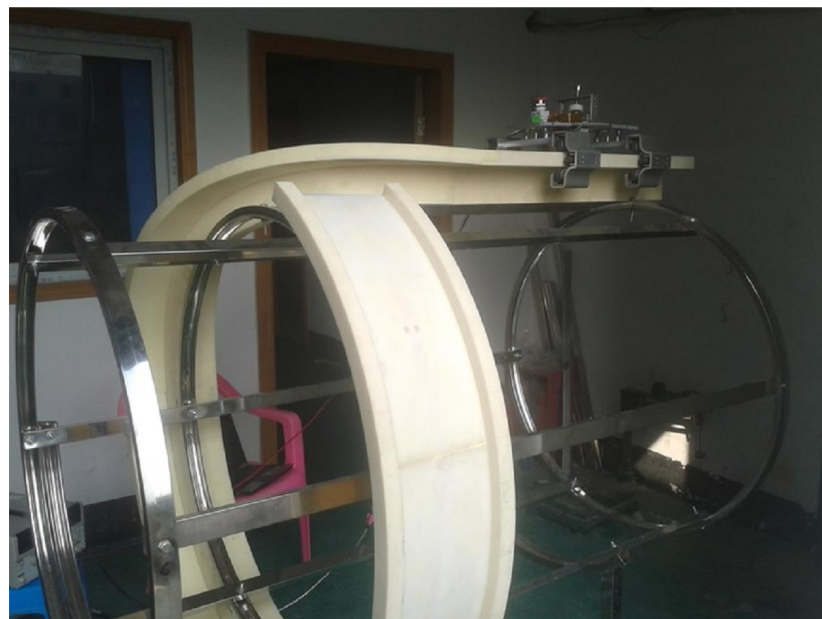
Fig. 2 Prototype of Circular-Rail Robot System (CRRS)
