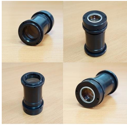
Fig. 2 – Optical system of star tracker experimental model
