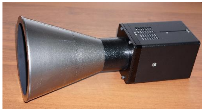
Fig. 4 - Experimental model of star tracker
