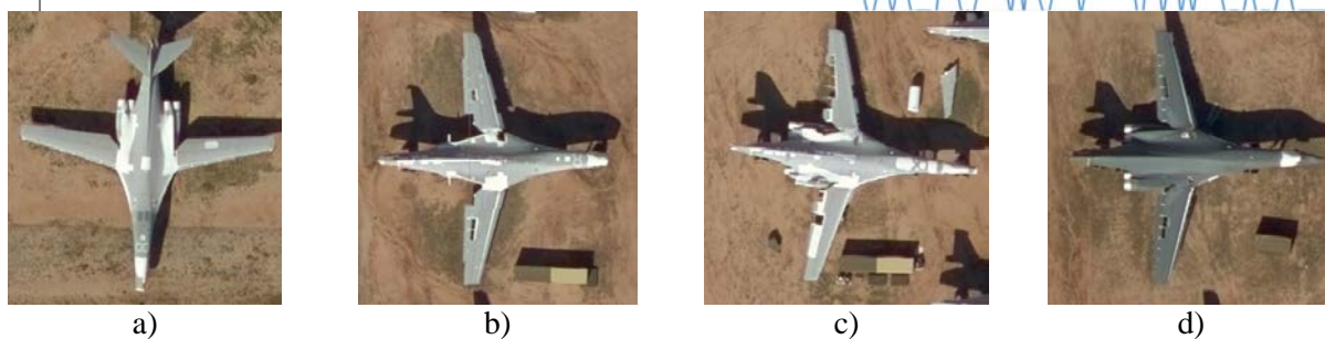
Figure 3. Instances of B-1 aircraft having various dismantled elements.
