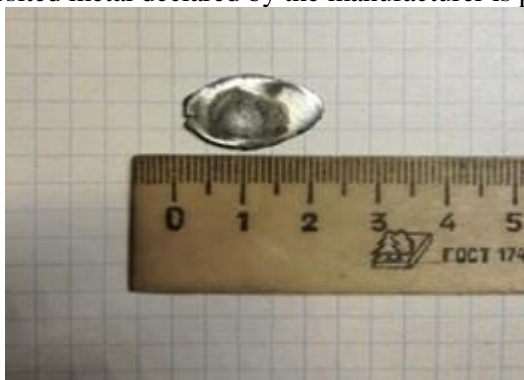
Figure 3. Sample after atomic-emission spectral analysis.
