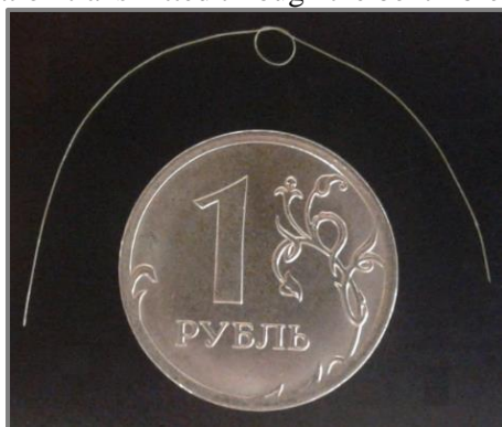
Figure 13. Example of possible curvature of the fibre with 110 µm in diameter (without shell).
