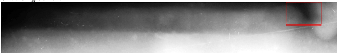
Figure 13. Image No. 2 of the radiographic image with the recognized defect “lack of fusion”.
