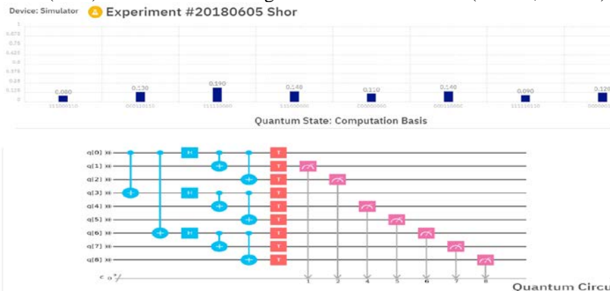
Figure 4. Encoding circuit for the Shor nine qubit code (Note: experiments of authors).
