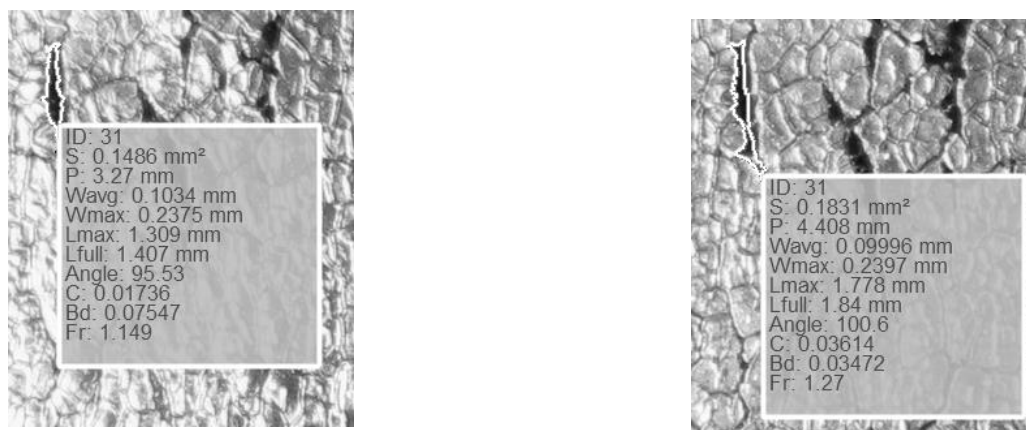
Fig. 6. An example of dynamic crack without merging with a difference of 3 days.
