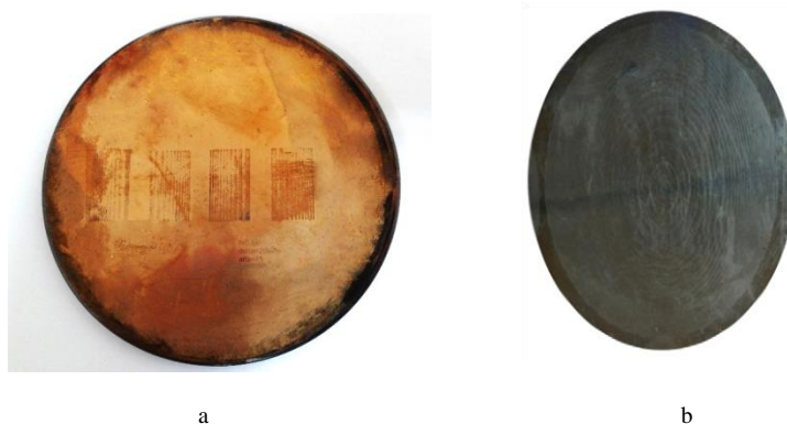
Fig. 1. The test objects: binary lens (a) and focuser to a point (b).
