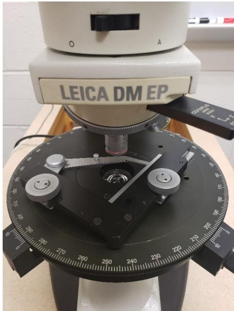
Figure 15. The graduated stage that was used during the point count analysis of the petrographic thin sections.
