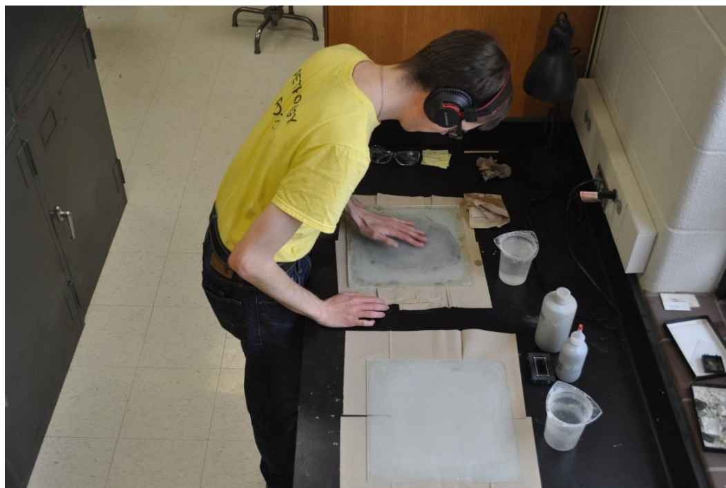
Figure 14. Hand grinding a thin section using different grades of silicon carbide grit, water and a glass plate.
