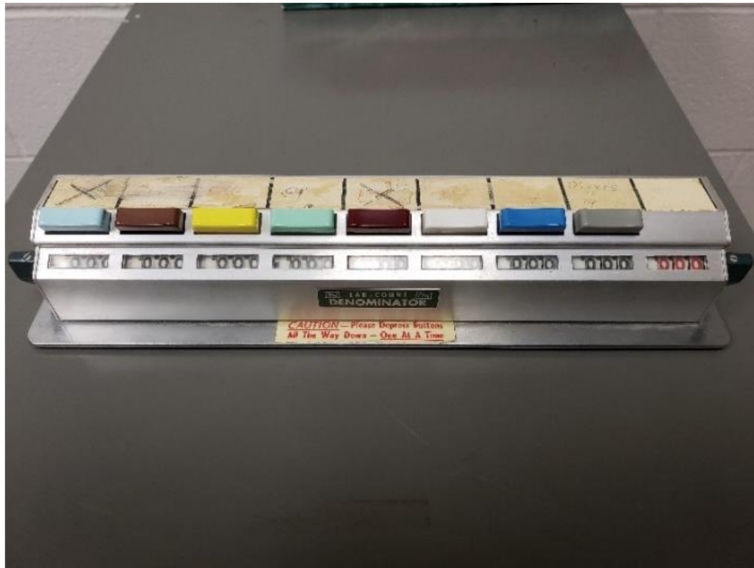
Figure 16. The Lab Count Denominator that was used to count the various amounts of minerals when performing the point count.
