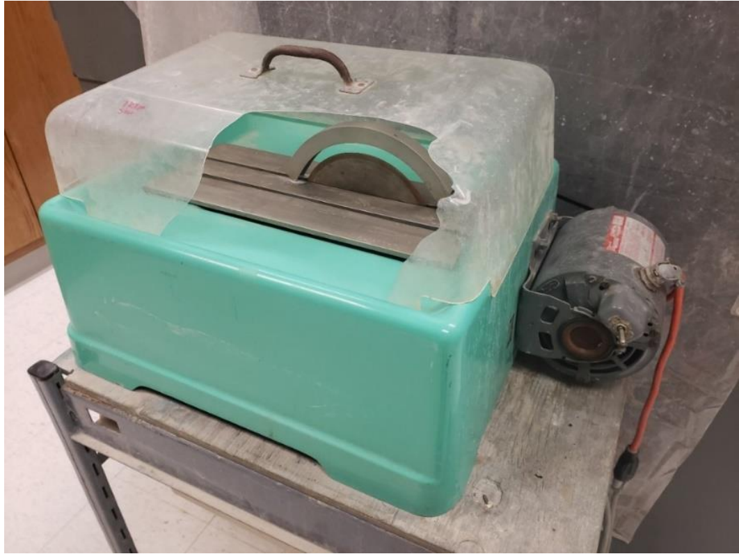
Figure 11. Water-cooled diamond blade trim saw used to cut bulk samples to appropriate size for thin section creation.
