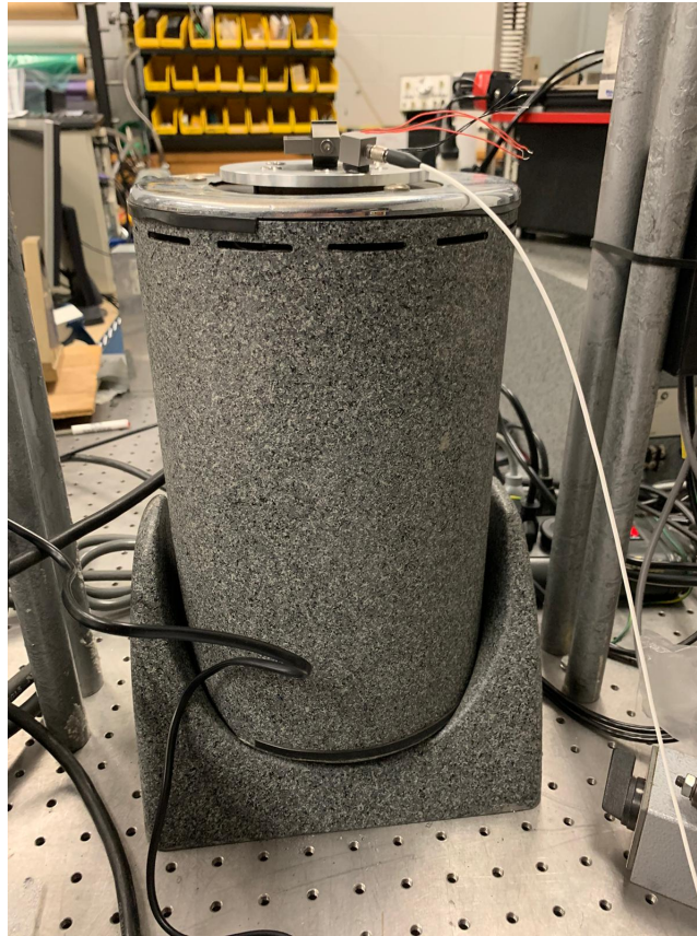
Fig. 16: Dynamic experiment setup of Flexensional Piezoelectric Energy Harvester
