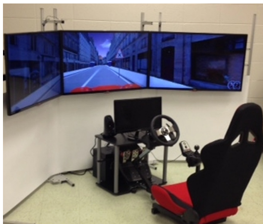
Fig. 1. National Advanced Driving Simulator (NADS) miniSim™ used in Experiment.
