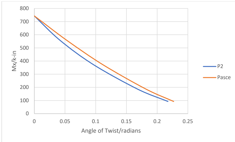
Figure 131. Moment vs Angle of Twist. Biaxial Bending. 8 in. x 8 in. x 3/8 in. Three Span
