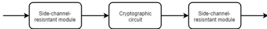
Fig. 4.1: Conceptual model of proposed comprehensive countermeasure to ML attacks and SCA attacks. Both ends of the cryptographic circuit is protected by a ML model. The uncertainty is retained by the keys stored/inserted on the cryptographic circuit.
